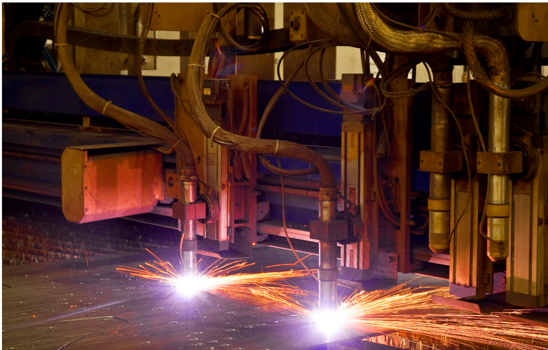
One of several MG burning machines with plasma capabilities
