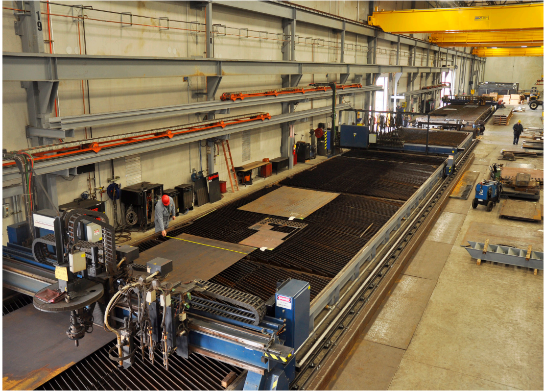
MG2- 2 Torch Plasma with 5-axis Bevel Head
