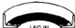
LEG IN Specify outside diameter and if unequal which leg is in
